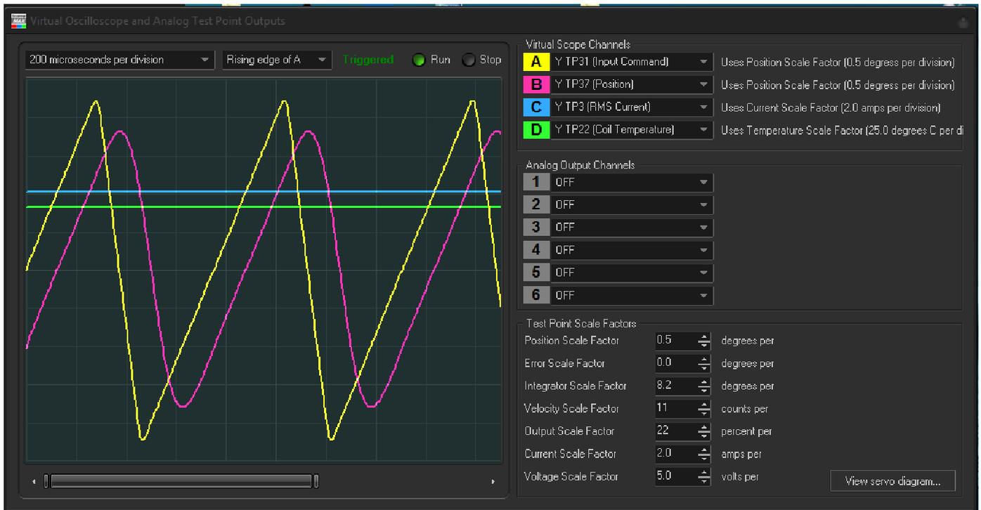
In this case we see that the RMS current being driven into the scanner is just above 4 amps, and coil temperature is still around 35C (assuming the scanner body is 30C). The scanner will be dissipating 16 watts, and power required from the power supply is around 2.25 amps per rail.
