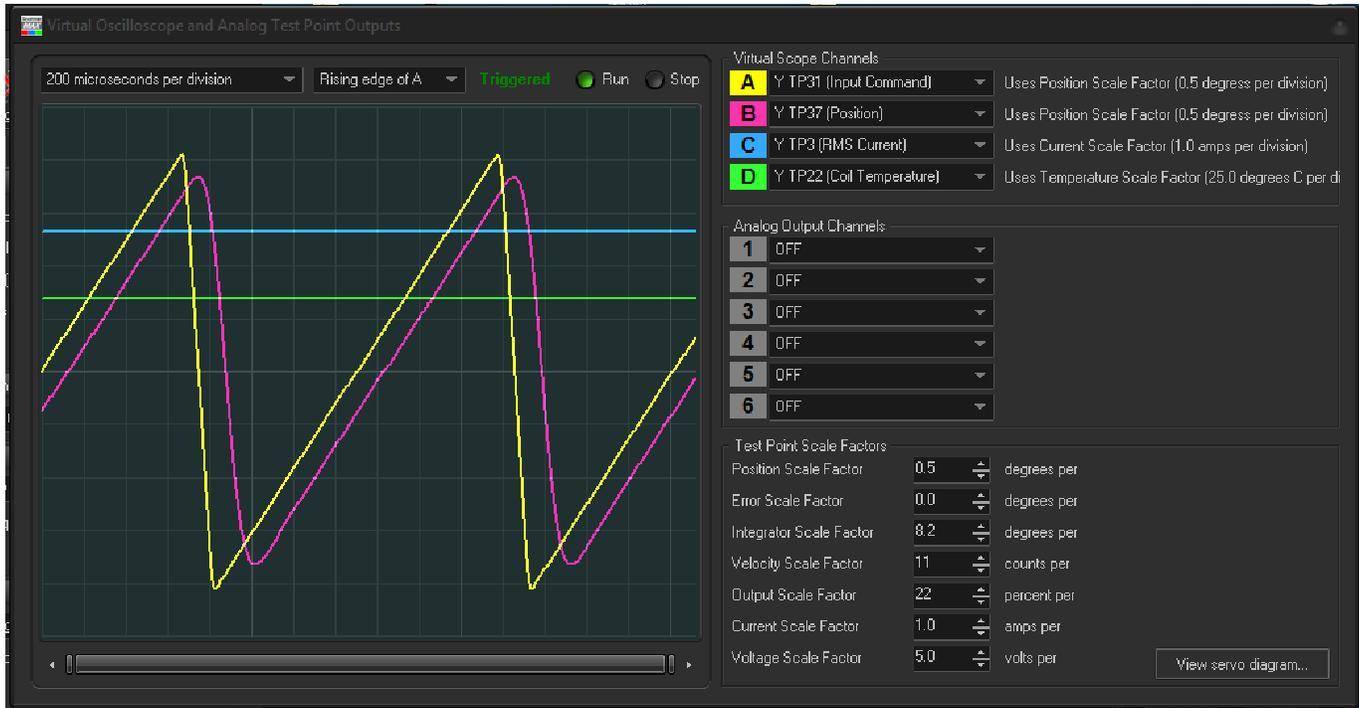
In this case, the coil current is 2.7 amps RMS and coil temperature is around 32 degrees C. The scanner will be dissipating 7.3 watts, and power required from the power supply is around 1.5 amps per rail.
