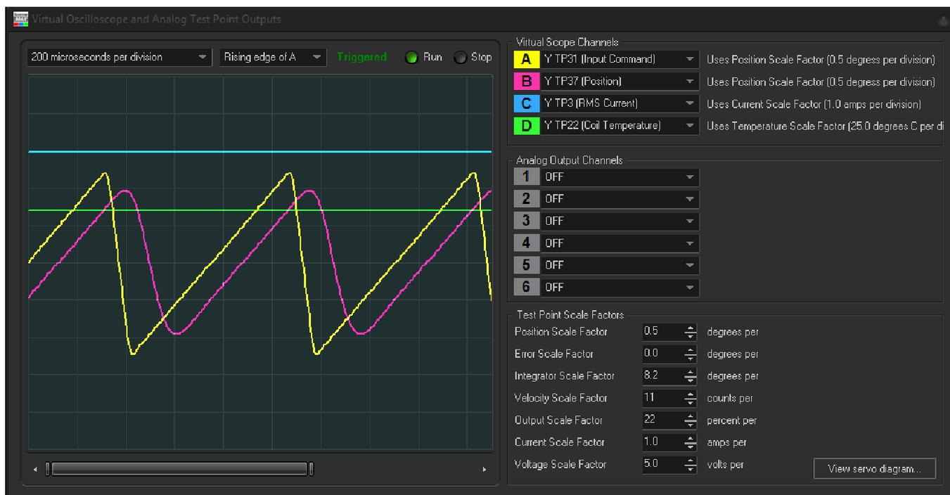
The oscilloscope shows that the RMS current being driven into the scanner is almost 3 amps and coil temperature is only around 35 degrees. Note that at this current, the scanner will be dissipating 9 watts of heat, which is certainly manageable. Power required from the power supply is around 1.8 amps from each of the +24V and -24V supply rails.
