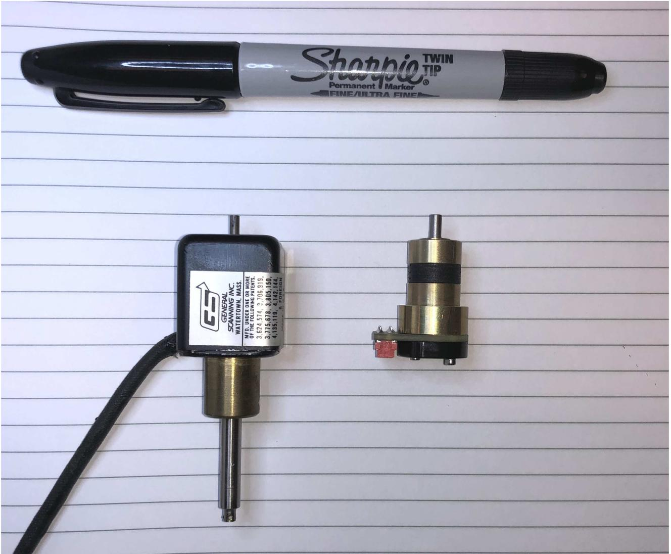
The compact 506 certainly occupies a smaller volume of space, and is lighter too. The General Scanning G-series of scanners is made primarily of iron, brass and copper, and weighs 75 grams. On the other hand, the Compact 506 is made primarily of aircraft aluminum, and weighs a bit more than 12 grams.
